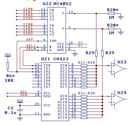
The OC pin of CH423 is a low-resistance open-drain output in the open-drain output mode. The on-resistance is
